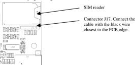
7. Connect power to the TS100. Once the LED's reach idle mode commands may be issued from the Teraterm window to the TS100. A programming session must always be started with entering of the programming password (default: admin). As long as programming continues there is no programming timeout in the system but once the TS100 has not received any commands in a period of approximately 5 minutes, entering the password will once again be required to continue programming.
